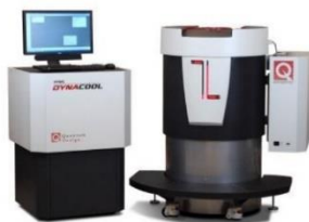
Quantum Design: PPMS DynaCool (Cryogen Free) Temperature Range: 1.8K - 400K Magnetic Field: \pm 14 T
